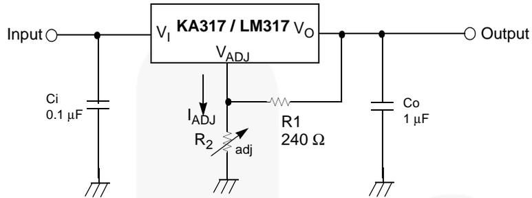
$$V_O = 1.25 \text{ V} \left( 1 + \frac{R_2}{R_1} \right) + I_{ADJ} R_2$$
