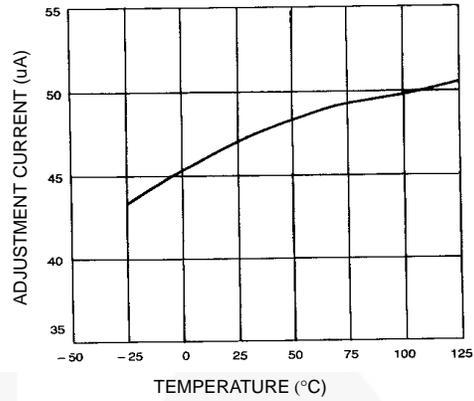
Figure 3. Adjustment Current
