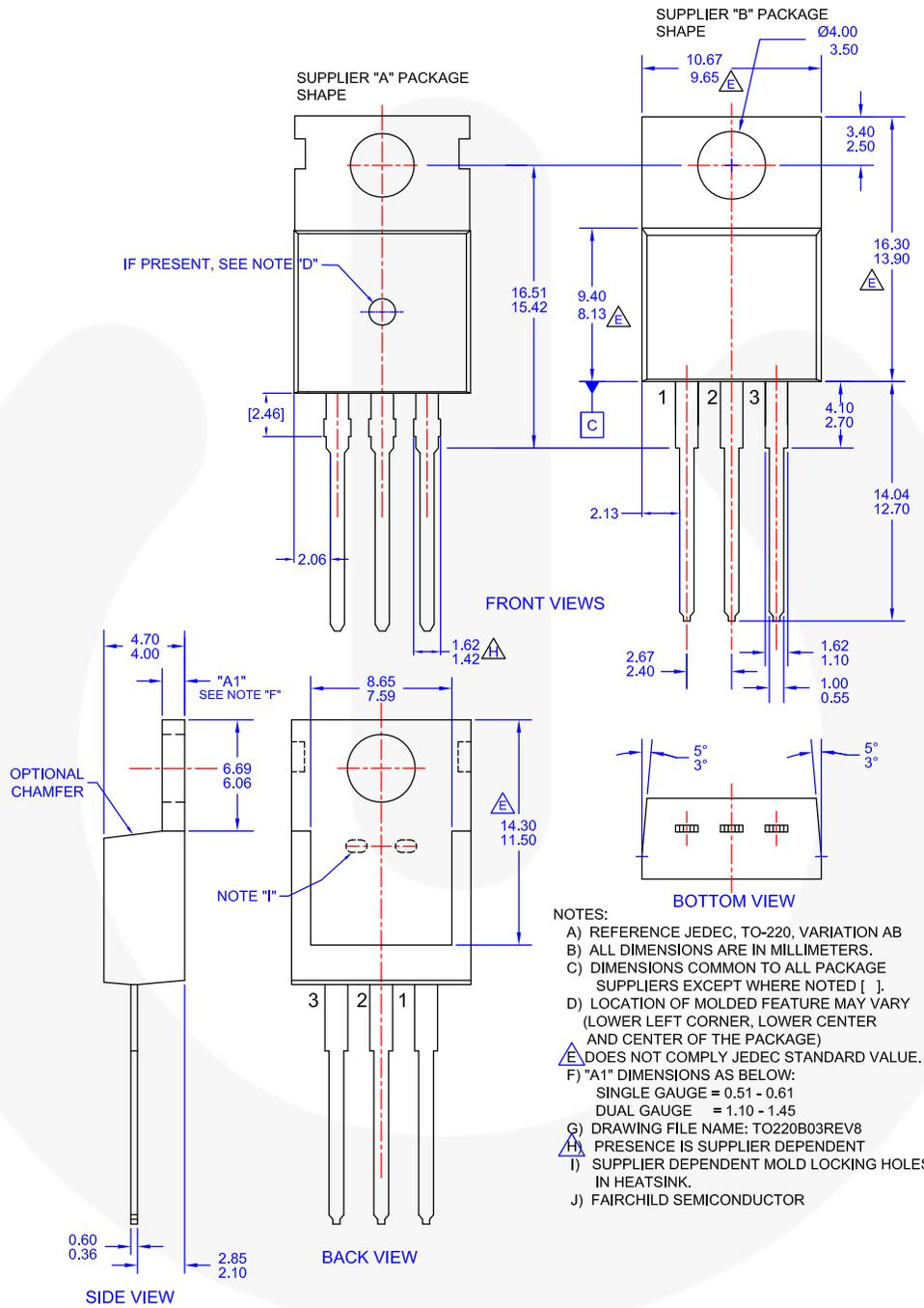
Figure 8. TO-220, MOLDED, 3LEAD, JEDEC VARIATION AB
